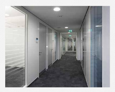
M100 is our modular partitioning system that can be used to form combination runs of both solid and glazed elevations, all utilising a common 100mm framework platform. This offers great flexibility, with simple adaptations enabling screens to be changed from glazed to solid, or vice versa. Our full range of deflection heads; ±15mm, ±25mm and ±40mm are compatible too, so there is no need to deal with those awkward detail junctions between a drywall crosswall andglazed room frontages.
