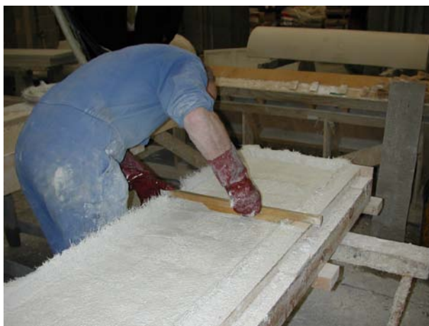
Figure 1.4 Gauging thickness of GRC
