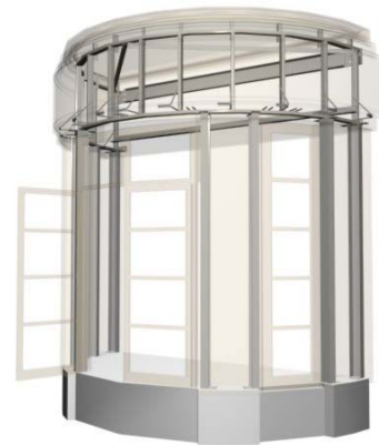
Figure 3.12 - Curved Stud Frame Panels for Portico Construction
