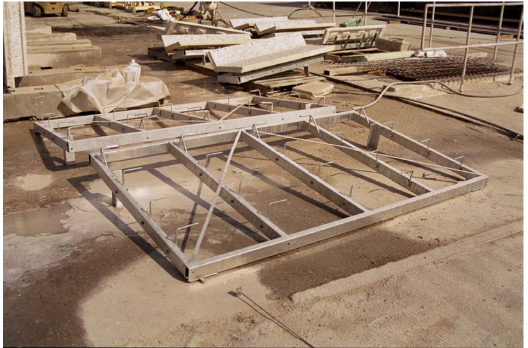
Figure 3.6 - Stud Frame fabricated from Rectangular Hollow Sections
