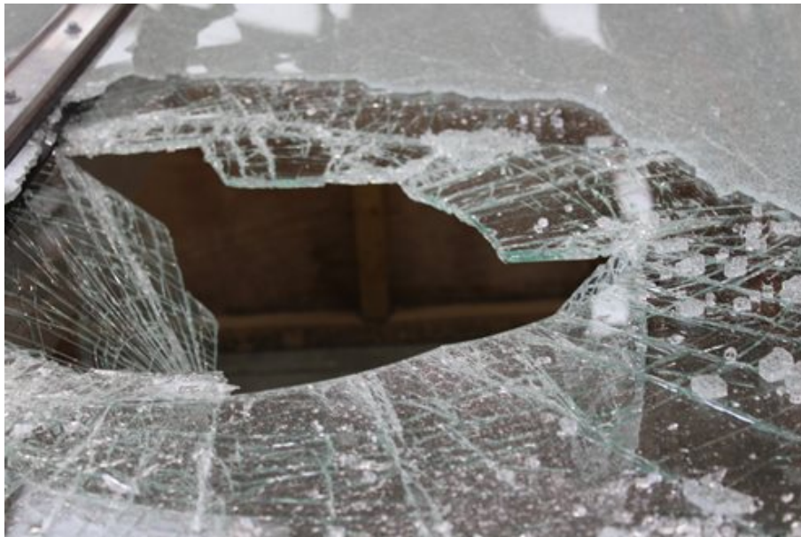
CWCT testing requires the outer pane to be broken and the test weight supported only on the inner pane for a successful pass.
