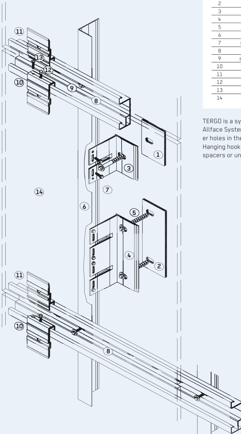
TERGO is a system for secret fixing EQUITONE panels (12mm) to the Allface System F1.44. The panels have factory drilled undercut fastener holes in the back of the panel.
