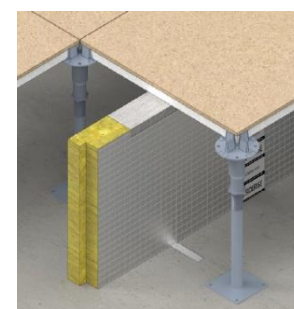
Fig 6. CVB with optional rebates and added stabilising brackets
