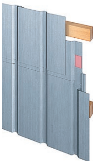
Longitudinal connection – slave profile for vertical application
