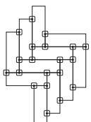
For herringbone designs, put FlexLok pads on each corner, adhesive side up.
