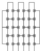
Lay the first row of planks and put FlexLok pads at each joint, adhesive side up. Install the remaining carpet tiles, placing FlexLok tabs as illustrated in the image.
