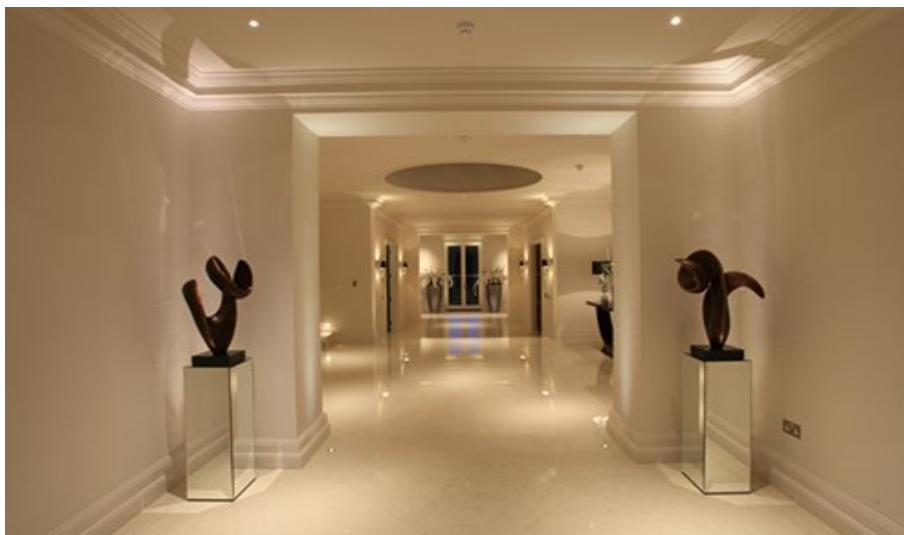
Avoid grids of downlights. Instead position them carefully to light your artwork, wash light down curtains or pinspot the centre of a coffee table.
