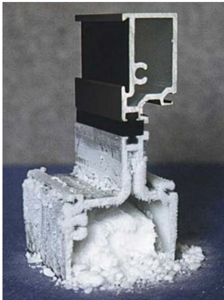
An example of the 'fill and de-bridge' design of thermal breaks which were introduced about 40 years ago.
