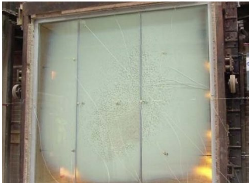
A frame and glazing under fire test - note how the glazing has become obscured by heat to reduce the transmittance of radiant heat.
