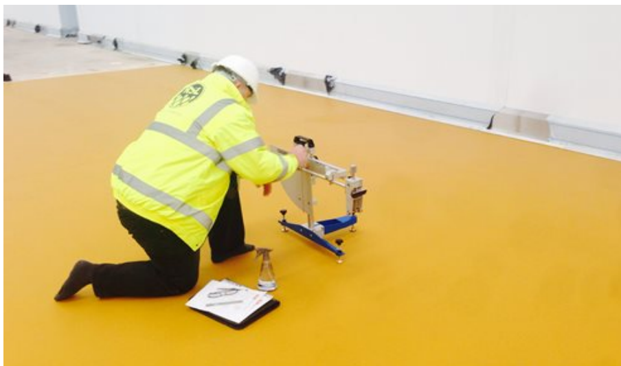
Non-slip performance testing on polyurethane floor screed using the TRRL Pendulum
