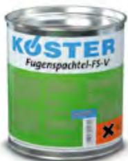
Formstable joint sealant with excellent resistance against mechanical stresses and a high resistance against water, sea water, salt solutions, petroleum and mineral oils. It is rot and root resistant. The rubber-elastic material based on polysulfides is 2-component, elastic and stable.
