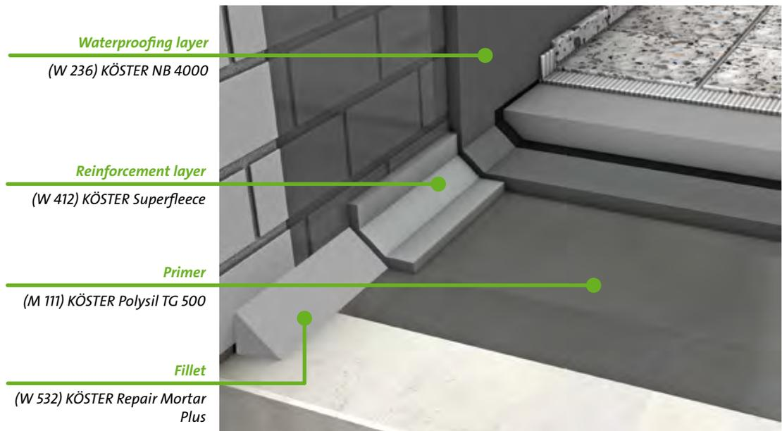
Balconies and terraces are constantly exposed to rain, splash water and high temperature fluctuations. Therefore the waterproofing should always be crack bridging.
