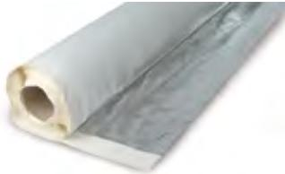
Cold applied self-adhesive rubber / bitumen sealing membrane for the waterproofing of small, weather exposed areas such as roofs, garages or balconies. Applicable between + 12 °C and + 35 °C.
