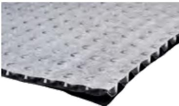
Green HD-PE based notched protection board which combines 3 functions in one product: (1) mechanical protection of the waterproofing layer (e.g. when backfilling the construction pit) according to the DIN EN 18533, (2) decoupling of the waterproofing layer from any ground movement, (3) the hollow core leads seepage and backwater safely to the drainage.
