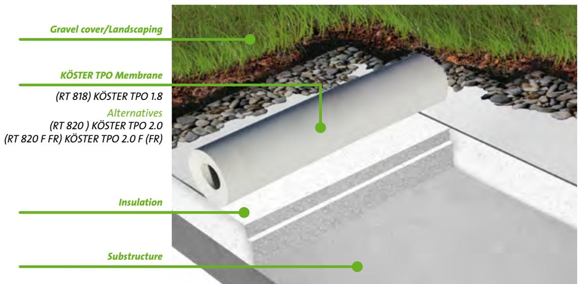
A quick and secure way to install KÖSTER TPO Membranes is through loose laying with ballast. Ballast can consist of either gravel, paving slabs, or even green roofs. Ballast helps protect the roofing membrane against wind loads and can accommodate a wide range of architectural styles. A special advantage of this installation method is
