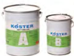
Fast setting vapor barrier for priming unsealed interior concrete floors under vapor tight flooring. Curing time 2-3 hours. The material reduces Moisture Vapor Emission Rates (MVER) and alkalinity to levels acceptable for most resilient or epoxy flooring systems as well as other vapor tight floorings such as sheet vinyl, VCT, rubber, wood, ceramic, sports, solid backed carpeting, epoxy, ESD and almost all other types of finished flooring.
