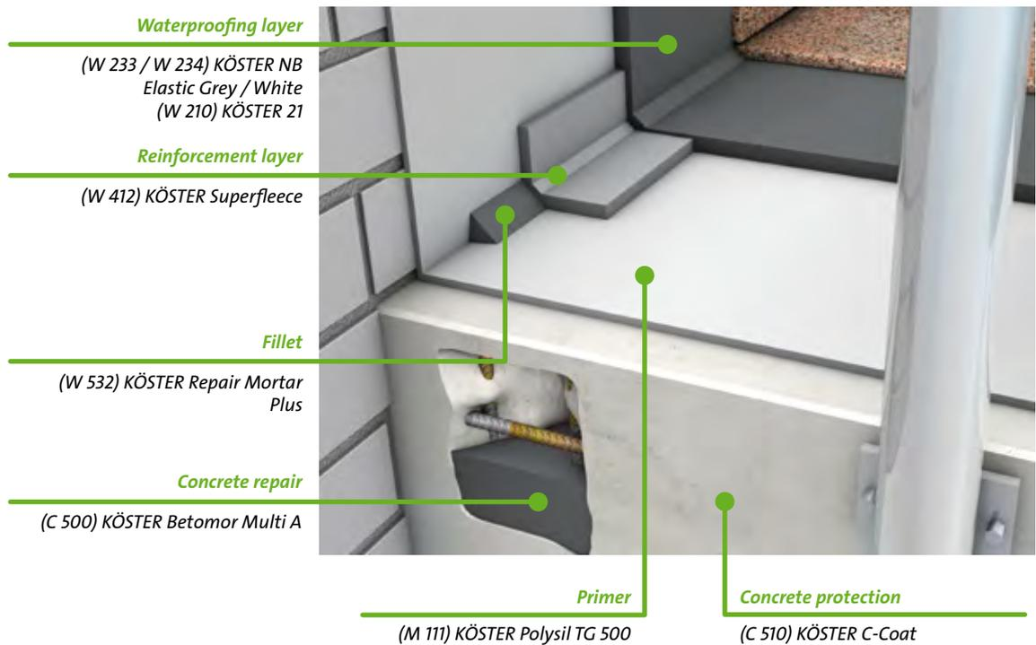
The mineral waterproofing of balconies and terraces is carried out with crack bridging KÖSTER NB Elastic (white or grey), or KÖSTER 21. This waterproofing is resistant to foot traffic and can be covered with tiles. It also bonds to damp substrates.
