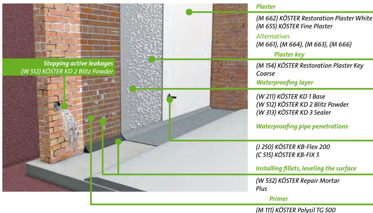
A very difficult situation: Basement waterproofing has to be done from the inside but water is actively entering the building. Often the only solution is the KÖSTER KD-System.
