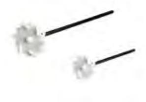
Special mixer for resins. Reduces air enclosures entrainment. Replaceable stirring disc. Shaft 12 mm Ø for chuck large version: hex head, stirrer diameter: 11 mm, stirrer length: approx. 48 cm, diameter stirring disc: 10 cm or 7.5 cm.
