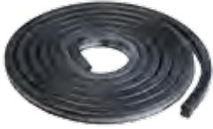
KÖSTER Quellband is a sodium-bentonite based water swellable joint tape with an alkalinity activated surface coating which stops premature swelling of the tape on the building site.
