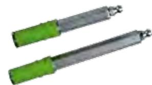
*KÖSTER masonry packer is particularly suitable for pressure injections into masonry. It provides a high and homogeneous contact pressure to the borehole. Four fins and two ridges on the rubber gasket prevent rotation during tightening and facilitate the optimal fixation of the packer in the borehole. It has a firmly mounted cone-head fitting for pressure injection and is galvanised.*
