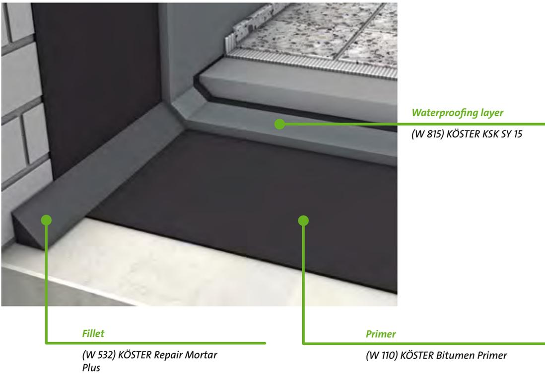
A fast and easy method for waterproofing balconies and terraces is using the cold applied self adhesive KÖSTER KSK waterproofing membranes.
