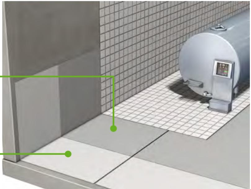
For the protection of concrete surfaces against acids the first step is to coat the surface with the negative side waterproofing KÖSTER NB 1 Grey or the faster version KÖSTER NB 1 fast. The acid protection itself is made with KÖSTER Silicate Mortar (also suitable for damp substrates) or KÖSTER PSM (suitable for dry substrates and easy to apply).
