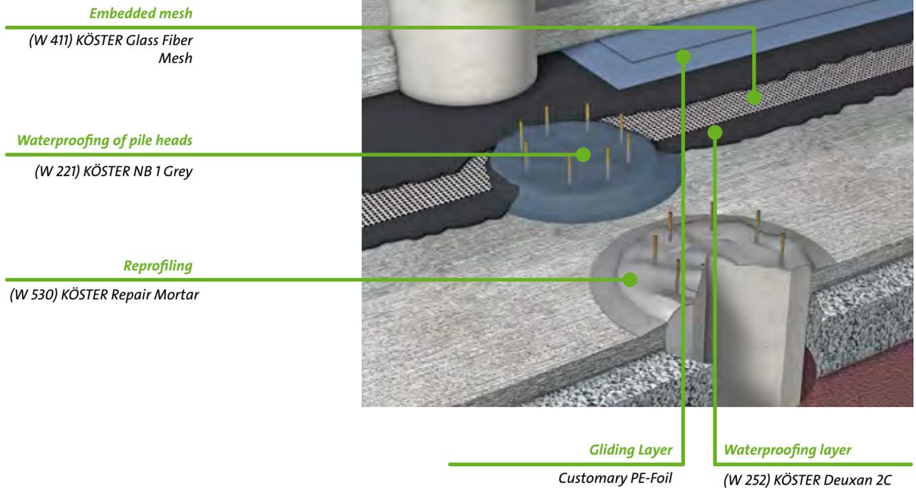
Damage in existing buildings is often caused by leaking pile foundations. Water can enter the building through the construction joints or it makes its way along the reinforcement steel. The waterproofing of pile heads has to withstand heavy loads from the whole building and it needs to be easily connected to the area waterproofing.
