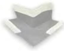
Ready to use, elastic moulded part for the waterproofing of outside corners in the KÖSTER BD System. Made of NBR-rubber with an protruding mesh for the secure integration into the area waterproofing. The KÖSTER BD System is a ETAG 022 certified system for the waterproofing of wetrooms e.g. under ceramic tile.
