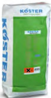
Injection grout for the restoration of structural strength in cracks or voids in masonry and concrete. KÖSTER Micro Grout 1C possesses a high compressive strength, is shrink free, and does not show sedimentation during its pot life. Fields of application include crack injection also in overhead areas, filling of voids, as well as the grouting of masonry anchors.
