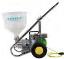
*Electrical pump for spraying liquid and pasty, mineral-, water-, or bitumen based materials such as 1 and 2 component polymer modified bitumen thick film sealants, elastic and rigid waterproofing slurries, liquid membranes, and mortars.*
