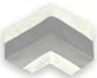
Ready to use, elastic moulded part for the waterproofing of inside corners in the KÖSTER BD System. Made of NBR-rubber with protruding mesh for the secure integration into the area waterproofing. The KÖSTER BD System is an ETAG 022 certified system for the waterproofing of wetrooms e. g. under ceramic tile.
