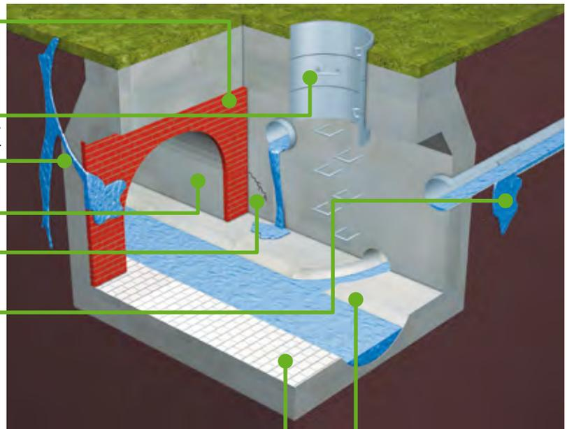
Water treatment facilities like sewage treatment plants, sewers and shafts or sewage water tanks made from concrete or masonry are exposed to a variety of stresses. The restoration of such facilities entails waterproofing, concrete repair and concrete protection as well as protection against acids and abrasion. For this a wide range of materials are used.
