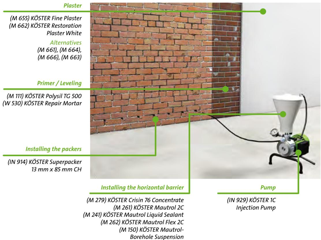
*Fast and effective: The installation of a horizontal barrier via pressurized injection. When it is possible to ensure that the wall is free of cracks or voids, the horizontal barrier can be installed with a pressurized injection system. Cracks and voids which become apparent during the drilling process can be filled with KÖSTER Borehole Suspension. After filling, the borehole is re-drilled.*
