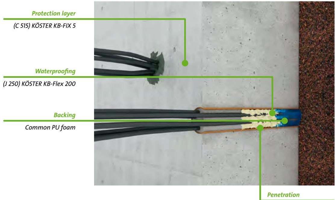
Cable and pipe penetrations such as electrical, water and data cables, must be permanently and securely waterproofed against penetrating water. Typically, rigid mortars or foams are used, which prevent the installation of other cables.
