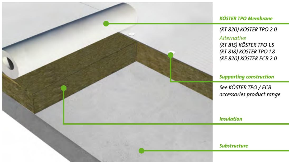
The most common method of installing TPO membranes is through mechanical fastening. The membrane is mechanically fastened to the roof structure, which can consist of either wooden sheathing, trapezoidal sheets, or a concrete slab. The membrane is generally fastened through the thermal insulation, which requires special fasteners.
