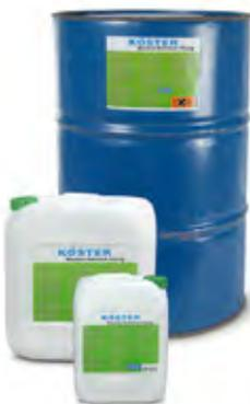
Very thin fluid, deeply penetrating silicifying concentrate for waterproofing against rising damp (wicking moisture) in masonry. It reacts to water insoluble and water-repelling compounds which also have a solidifying and strengthening effect on the building material. Together with KÖSTER NB 1 Grey and KÖSTER Restoration Plasters it is suitable for the restoration of masonry.
