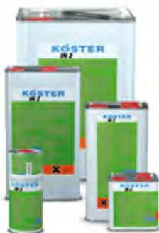
Elastic PU injection resin. For permanently waterproofing cracks and joints. It is designed to withstand continuous contraction and expansion and is therefore ideal for the repair of moving cracks. Also suitable for slightly damp cracks. Viscosity approx. 200 mPa.s.
