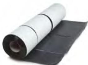
Cold applied self adhesive rubber / bitumen based waterproofing tape for sealing facade areas and windproofing window connections. Applicable between + 5 °C and + 30 °C. Highly flexible, crack bridging immediately water and rainproof. Double laminated with a highly tear resistant polyethylene foil.
