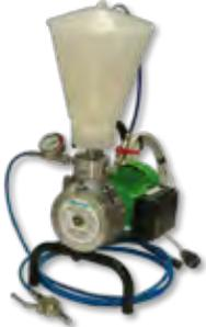
Electrical 1C injection pump for injecting of cracks and voids. It is suitable for the injection of all KÖSTER injection materials (foams and resins). Operating pressure can be adjusted from 0 - 200 bar. The maximum delivery rate is approx. 2.2 l / min.
