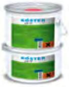
KÖSTER ESD 175 is a water based epoxy dispersion for priming floors to be coated with KÖSTER ESD 275. The KÖSTER ESD System creates an ESD protected area according to the norms DIN EN 61340 and DIN EN 61340-1, supplementary sheet.
