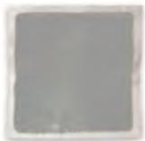
Ready to use, elastic moulded part for the waterproofing of floor drains in the KÖSTER BD System. Made of NBR-rubber with an protruding mesh for the secure integration into the area waterproofing. The KÖSTER BD System is a ETAG 022 certified system for the waterproofing of wetrooms e.g. under ceramic tile.
