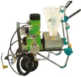
Electrical 2C injection pump with stageless adjustable mixing ratio (gel : water). Operating pressure is approx. 30 bar. The maximum delivery rate is approx. 2.5 l / min.
