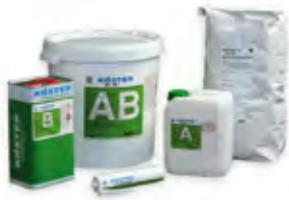
Self leveling floor coating with high chemical resistance and high abrasion resistance. Food safe and resistant against temperature shocks. Three component polyurethane cement floor coating. KÖSTER UC 100 is applied in a layer thickness between 3 and 9 mm.
