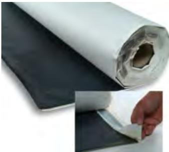
Cold applied self-adhesive rubber / bitumen waterproofing membrane according to the DIN EN 18533. Suitable for application from + 5 °C to + 30 °C. Fields of application include basements, foundation plates, balconies, terraces or on polystyrene elements.
