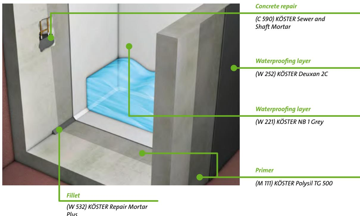
Concrete water tanks are waterproofed from the inside using KÖSTER NB 1 Grey. KÖSTER NB 1 Grey is certified for use in drinking water environments.
