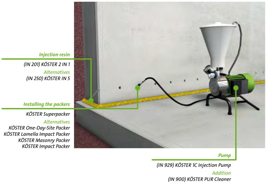
For retroactive waterproofing of the wall-floor junction the boreholes have to be drilled transecting the construction joint. The borehole should be drilled approximately into the middle of the construction joint.
