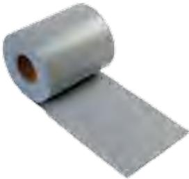
Thermoplastic tape for sealing expansion and dilatation joints (up to 12 cm) and broad, irregular cracks. KÖSTER Joint Tape 20 is UV resistant, highly elastic and can withstand extreme movements in the joint. The joint tape system consists of KÖSTER Joint Tape and KÖSTER KB-Pox Adhesive, a high performance adhesive for fastening the joint tape to mineral substrates. 1 mm x 200 mm.
