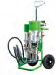
*Pneumatic pump made of stainless steel for the application of KÖSTER Injection Gel G4. Mixing ratio 1:1 Capacity: Max. 11 ltrs. per minute. Working pressure: 20 - 200 bar.*
