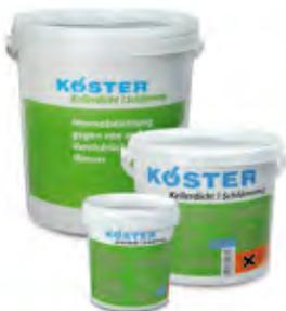
Fast setting, mineral sealing slurry with high resistance against aggressive ground moisture and pressurized water. Used in combination with KÖSTER KD 2 Blitz Powder and KÖSTER KD 3 Sealer for the negative side waterproofing of mineral surfaces such as in internal basement waterproofing. The KÖSTER KD System stops flowing water and forms a permanent waterproofing layer on masonry and concrete.
