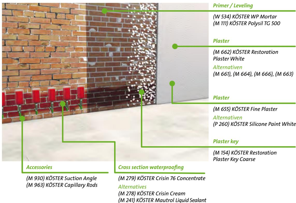
Rising (or “wicking”) moisture is among the most frequently encountered causes of damage in masonry walls. The results are clearly identifiable through the spalling of plaster, damaged joints and bricks, and also through salt efflorescence and algae growth. Damage from rising moisture can be avoided by the installation of a horizontal barrier.
