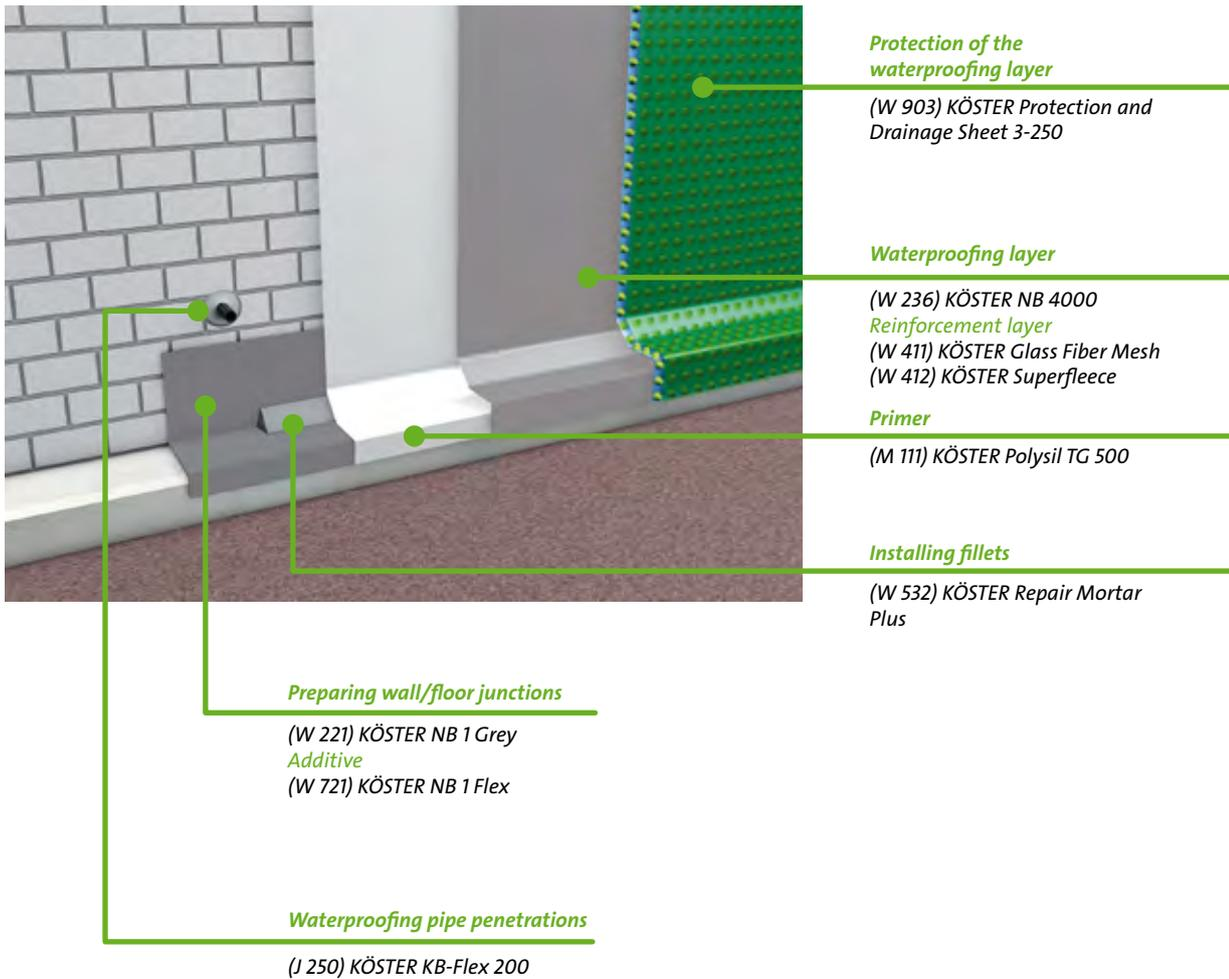
Mineral sealing slurries are especially robust waterproofing systems with extremely good adhesion to mineral surfaces. They are not affected by moist surfaces and become an integral part of the building structure on which they were applied. Mineral sealing slurries are paste-like and are applied seamlessly to the building element being waterproofed. They are easy and safe to apply and can be installed as a rigid or crack bridging system.
