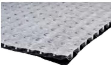
Black HD-PE based notched protection board which combines 3 functions in one product: (1) mechanical protection of the waterproofing layer (e.g. when backfilling the construction pit) according to DIN 18195, (2) decoupling of the waterproofing layer from any ground movement, (3) the hollow core leads seepage and backwater safely to the drainage.
