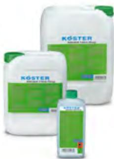
Low viscosity silicifying liquid. The active ingredients penetrate deeply into the substrate and form water insoluble compounds. The pores are plugged and permanently waterproofed through continuing crystallization. Used in combination with KÖSTER KD 1 Base and KÖSTER KD 2 Blitz Powder for the negative side waterproofing of mineral surfaces such as for internal basement waterproofing. The KÖSTER KD System stops flowing water and forms a permanent waterproofing layer on masonry and concrete.
