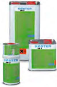
Viscoplastic 2- component PU injection resin for the restoration of structural strength in cracks and joints. Solvent free, low viscosity. Compressive strength  $\geq 80$  N/mm<sup>2</sup>, tensile strength 14 N/mm<sup>2</sup>.
