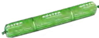
Highly elastic, low modulus polyurethane sealant, with good UV resistance and excellent adhesion to typical construction materials. KÖSTER PU 907 is one component and cures with moisture to form a flexible sealant which can be overpainted after curing is finished. The sealant is non sagging, highly thixotropic, easy smoothing and has good workability.
