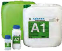
Low viscosity acrylic gel for curtain injection and area injection of masonry. Water based, elastic gel with a very low starting viscosity after initial mixing. It is capable of binding water during gelation. The swelling ability after full curing allows a 40% uptake of additional water into the gel structure. Due to the low starting viscosity it can be injected into fine substrate pores. Drinking water certification.
