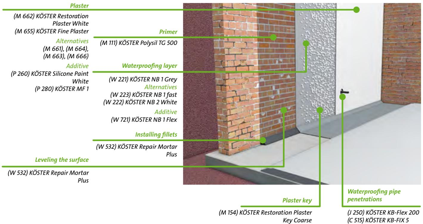
Retroactive waterproofing in existing buildings needs to be done with mineral waterproofing systems. They have excellent bonding characteristics to mineral surfaces and also won't detach from wet and moist substrates.
