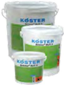
Shrink-free, fast curing multi purpose mortar for concrete restoration. In particular suitable for the protection of exposed reinforcement steel: It unites corrosion protection, coarse mortar, fine filler and bonding bridge in one product. For layer thicknesses from 0 – 60 mm.
