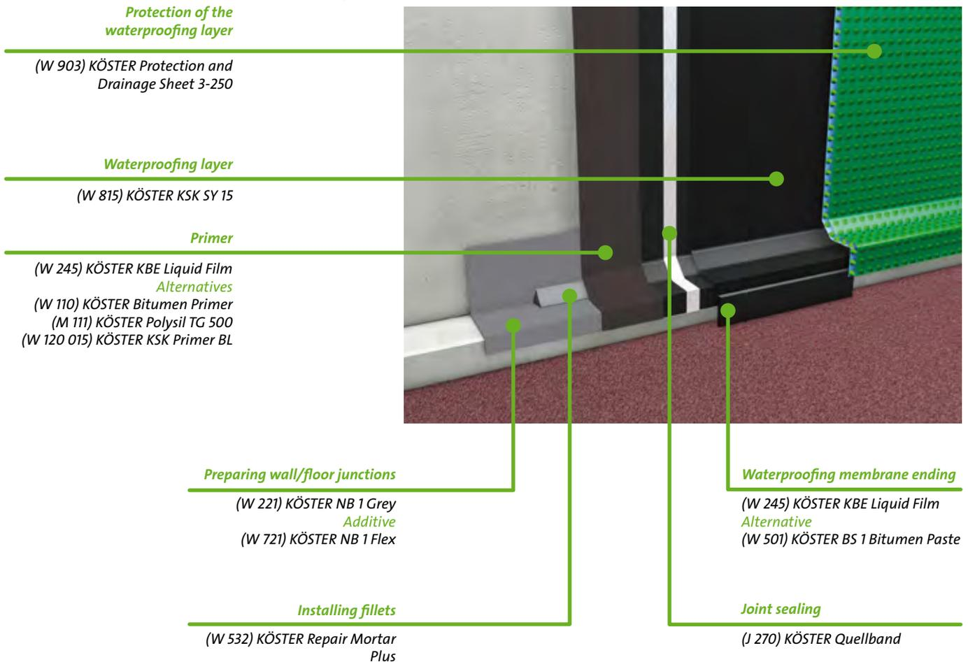
*Fast, clean, and easy: Exterior basement waterproofing with KÖSTER KSK cold applied, self adhesive waterproofing membranes. No drying time, instantly watertight, with a tight control of consumption.*
