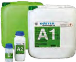
Reaction time adjustable acrylic gel for curtain and area injection, as well as filling voids. High adhesion to mineral substrates. Water based gel with low initial viscosity and elastic end properties. Can bind water during the reaction. Swells up to 10 % during hardening, and is reversible. Due to the low viscosity it can be injected into very fine pored structures using a multi-stage injection technique fitted to the reaction-time curve of the material.
