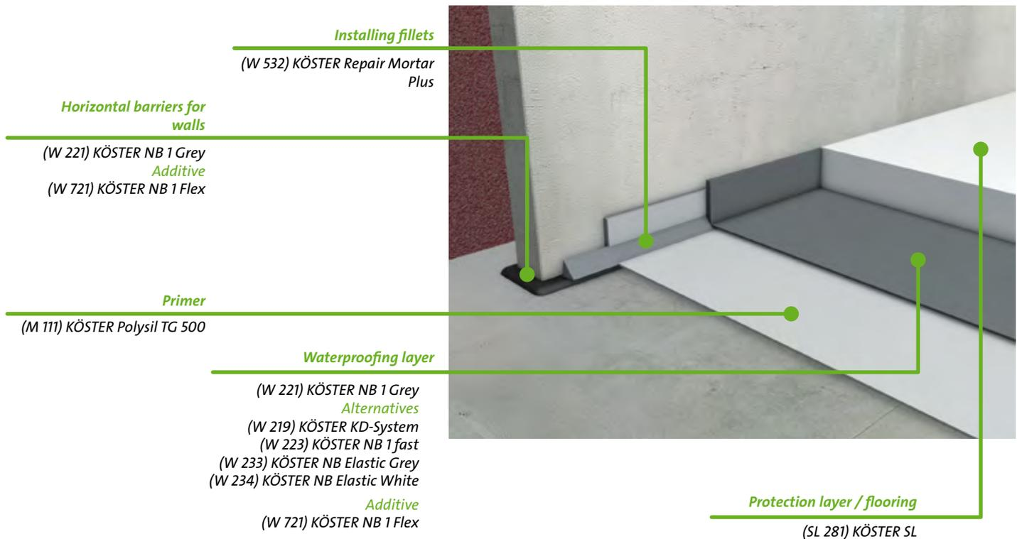
Mineral waterproofing systems have the advantage of excellent bonding properties of the waterproofing material to mineral substrates, the bond between the individual waterproofing layers is excellent too.
