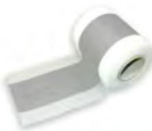
Joint sealing tape for the secure bridging of joints, wall-floor junctions and in areas prone to cracking. Specially designed for the KÖSTER BD System. An elastomer strip with protruding mesh for the secure integration into the area waterproofing. The KÖSTER BD System is an ETAG 022 certified system for the waterproofing of wetrooms e. g. under ceramic tile. 0.6 mm x 120 mm.
