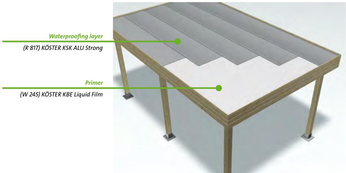
*Smaller roofs on non residential buildings can quickly and easily be waterproofed with the cold self-adhesive sealing membrane KÖSTER KSK ALU Strong. The clean and dry substrate is primed with KÖSTER KBE Liquid Film. KÖSTER KSK ALU Strong is applied onto the dry and primed roof area. Membranes have to overlap*
