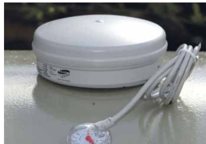
A typical tank telemetry unit
