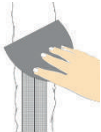
7. Bed scrim cloth over all joints (both walls & floors) using the tile adhesive to provide extra reinforcement.
