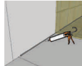
6. Run a bead of silicone along the internal joints before tiling and then again after the tiles are fitted - this is standard fitting procedure. (Tanking recommended when tiling wet rooms.)
