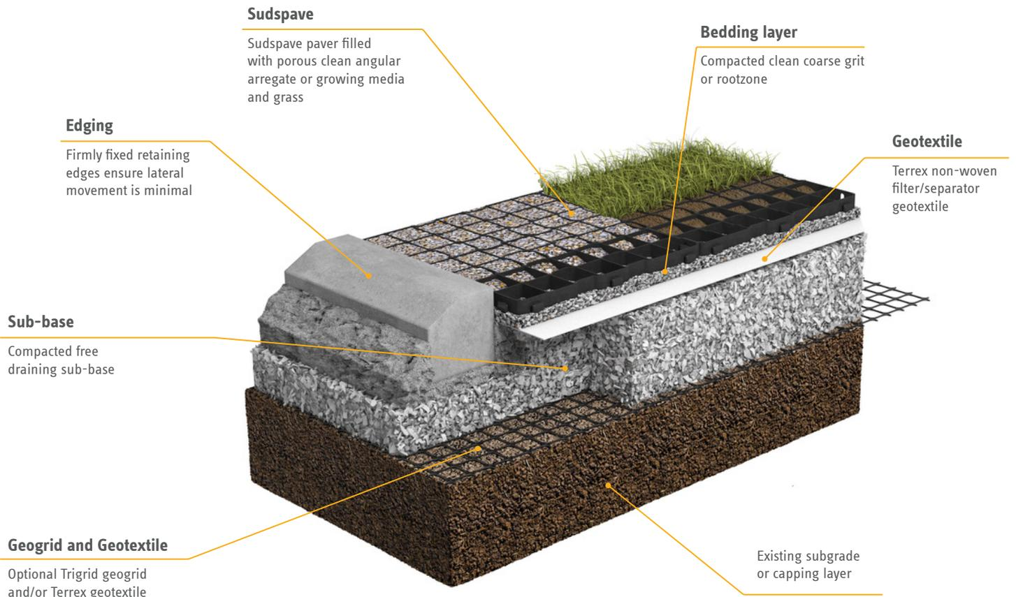
Infiltration option shown but containment option also available. Sub-base depth of both may be reduced by use of Abweb.
