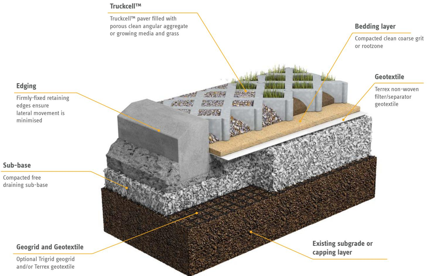
Infiltration option shown but containment option is also available. Sub-base depth of both may be reduced by use of Abweb.
